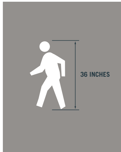
Pedestrian pavement marking
